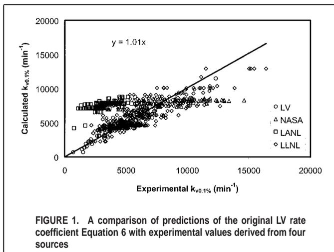
FIGURE 1. A comparison of predictions of the original LV rate coefficient Equation 6 with experimental values derived from four sources
