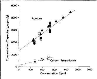
FIGURE 2. Linearized Langmuir isotherm plots for Willson (O) and Pulmosan ( $\Delta$ ) cartridges with acetone and carbon tetrachloride. Open symbols = dried; solid = as received.
