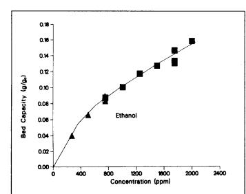
FIGURE 1. Adsorption isotherm plot of ethanol capacities from breakthrough curves for Willson  $(\bigcirc)$ , Pulmosan  $(\triangle)$ , and Norton  $(\square)$  cartridges. Open symbols = dried; solid = as received.
